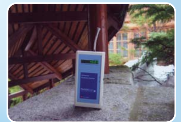
Particle test in Canada outdoors (Particle Level: 4,604 particles/ litre)
